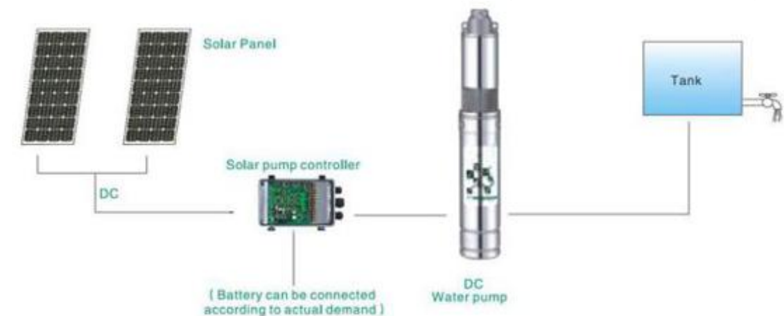
■ Working diagram of DC solar water pump system
